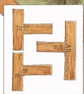
Each piece was marked to show its position. Then the frames were taken apart to be reassembled at the site.
