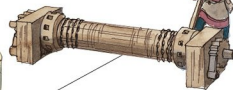
The winch gear that lifted the portcullis was operated by the guards. A brake on the side could be knocked out quickly to drop the barrier on intruders below.
