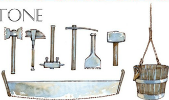
Masons' tools (left to right): picks and axes for quarrying and shaping stone; hammer and
