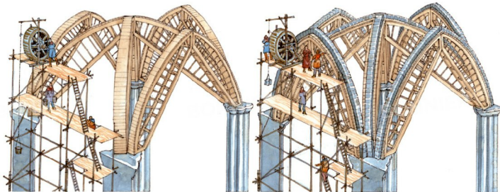
Stages in building a rib-vaulted roof are shown here. First, a wooden framework (called 'centring') was made and put in position.
