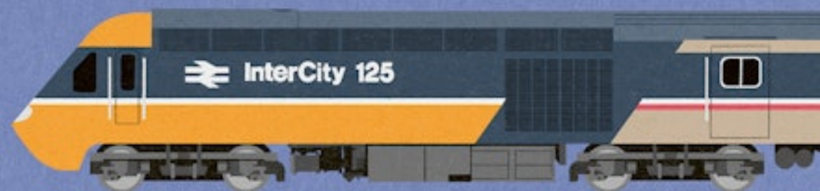
The InterCity 125 is one of the most successful diesel trains of all time. So named because it was designed to cruise at 125 mph (about 201km/h) when in service, it also holds the all-time speed record for diesel trains of 238km/h, which it reached in 1987.
