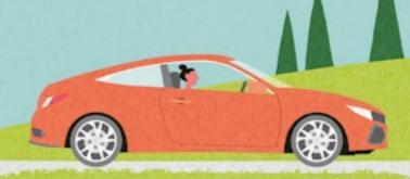
Coupes are sportier than a saloon. They usually have a fixed roof (unlike a convertible), a rear that slopes down, two doors, and seats for four people. 'Coupe' comes from the French word couper, which means 'out', reflecting the idea that this car type is a shorter, or 'out down', version of a more standard design.
