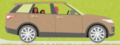
SUVs (or 'sports utility vehicles') can seat up to seven people. They're usually four-wheel drive, which means power from the engine is sent to all four wheels. SUVs also have high **suspension** to provide extra ground clearance, and are designed to drive comfortably over rough terrain.
