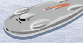
Silver, streamlined and sleek, the Railton Special looks like something from a science fiction film. In 1939, this 3-ton, 8.4m-long automobile powered by two supercharged Napier Lion W12 aeroplane engines, reached 695km/h on the Bonneville Salt Flats in the USA. The Railton Special and British driver John Cobb held the record for another 25 years.
