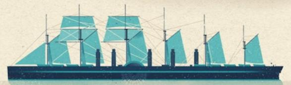
SS Great Eastern was a true giant of its day, designed by Brunel to carry up to 4,000 passengers non-stop between Britain and Australia. Launched in 1858, this 211-metre iron behemoth was powered by sail, the largest set of paddlewheels at that time and a screw propellor. Brunel died aged 53 only a few days after SS Great Eastern's first sea trial.
