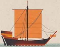
Used widely in the seas of northern Europe, cogs were sturdy and reliable cargo vessels, capable of carrying much more than the smaller knarr. Powered by a single square sail and steered with a rudder, cogs were more manoeuvrable than their tubby shape made them appear, and they could navigate the open sea as well as traverse wide rivers to reach inland ports.
