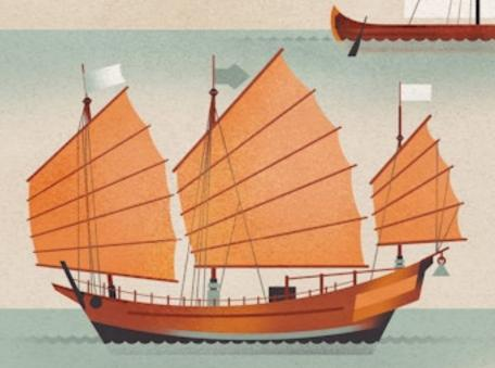
Invented in China during the 2nd century CE, junks are large wooden ships that are still used today. The first junks were sail-powered and used for transport, trade and warfare whereas modern junks have engines and are used for transport and leisure trips. Their wedge-shaped prows, wide hulls, tall sides and flat bottoms allow junks to navigate shallow waters as well as the high seas.
