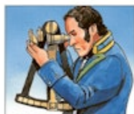
Officers use a sextant to measure the position of the sun and stars to find the ship's position.
