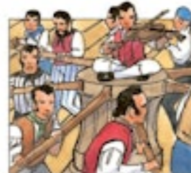
Crew use the huge capstan to wind the heavy ropes used for mooring and anchoring.
