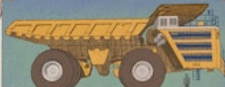
(2014) TYPE: Haul truck COUNTRY: Belarus LENGTH: 20.6 m The world's biggest mining truck hauls loads of metal ore weighing more than 40 tonnes from open cast mines. Temperatures in the mines can range from -50°C to +50°C.
